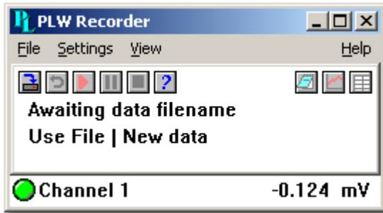
12. Connect a suitable voltage (for example, from a 1.5 V battery) to the channel. Pin connections are marked on the logger and also listed in the [Analog connector](#) topic.
