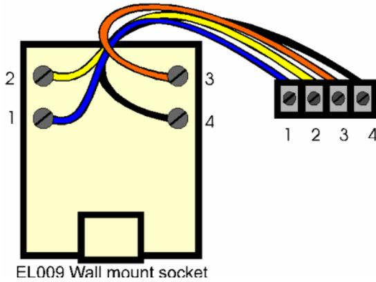
Connect adjacent units using four core cable, such as WI003. Connect terminal 1 to terminal 1, terminal 2 to terminal 2, and so on. The signals associated with each connection are as follows:
