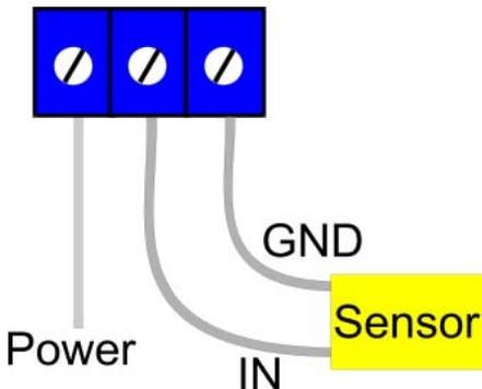
When measuring 4-20 mA with the EL037 supplying loop current, the transmitter should be connected like this:
