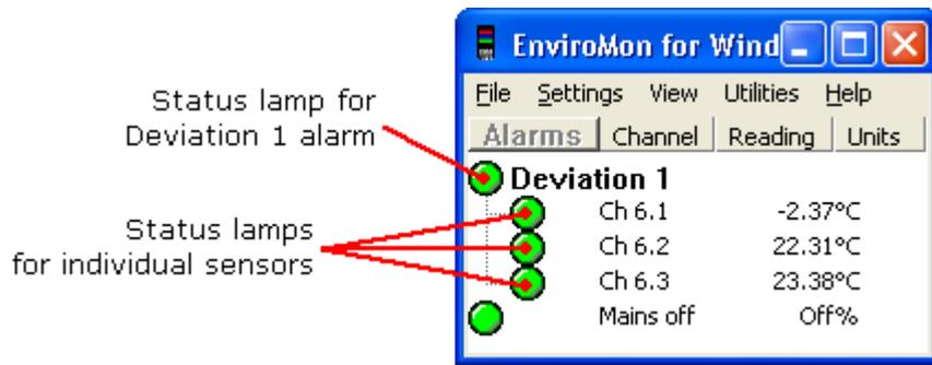
In this example, the monitor window shows that a deviation alarm called "Deviation 1" has been set up for the Ch 6.1, Ch 6.2 and Ch 6.3 sensors. The deviation alarm has its own status lamp, in addition to the lamps for the individual sensors.
