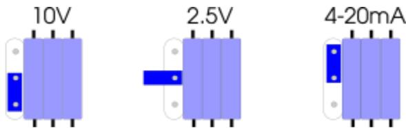
When measuring voltages, or for measuring 4-20 mA with the transmitter supplying the loop current, the input is connected between IN and GND. The PWR connector can be used to supply power to the transmitter:
