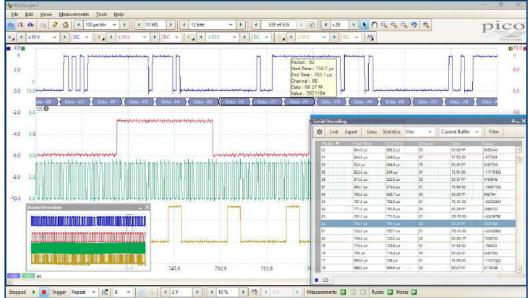
Table format shows a list of the decoded frames, including the data and all flags and identifiers. You can set up filtering conditions to display only the frames you are interested in or search for frames with specified properties.
